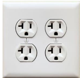
Quadplex 20-amp outlet. Each side should be labeled if separate circuits. Left side on one circuit (one cord), right side on another circuit for the second cord.
