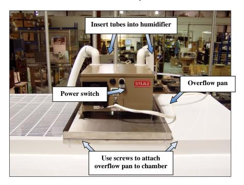
Next, connect the water line to the humidifier and to the water line hand valve. To connect the water line to the hand valve, simply insert the tubing into the compression fitting as far as it will go. If it becomes necessary to remove the tubing, press inward on the ring surrounding the tubing and pull the tubing outward. Next, connect the humidifier power plug to the receptacle located on the side of the chamber.
