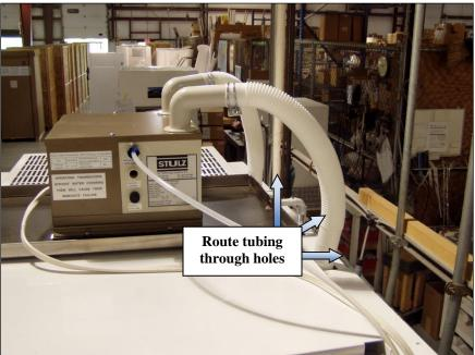
Next, install the ultrasonic humidifier and overflow pan on top of the chamber. The humidifier overflow pan should be attached to the top with the screws provided. Holes have been pre-drilled for attaching the overflow pan. Ensure that the humidifier power switch is in the 'On' position.
