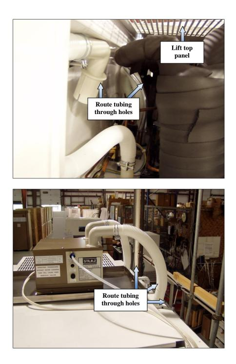
Next, install the ultrasonic humidifier and overflow pan on top of the chamber. The humidifier overflow pan should be attached to the top with the screws provided. Holes have been pre-drilled for attaching the overflow pan. Ensure that the humidifier power switch is in the 'On' position.
