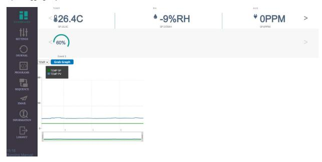
On the top is a carousel comprising of each of the sensors on the chambers. Each sensor has a block dedicated to it.
